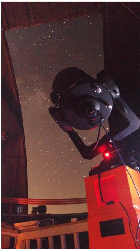
Figure 2: RHO 14" telescope, which will be roboticized for student use from campus.
